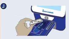
Open the drawer and place the test cassette into the holder as indicated, ...
