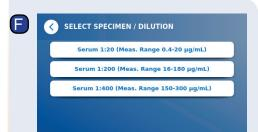
Some test methods may require a seleca tion of the specimen type and/or the sample dilution.
